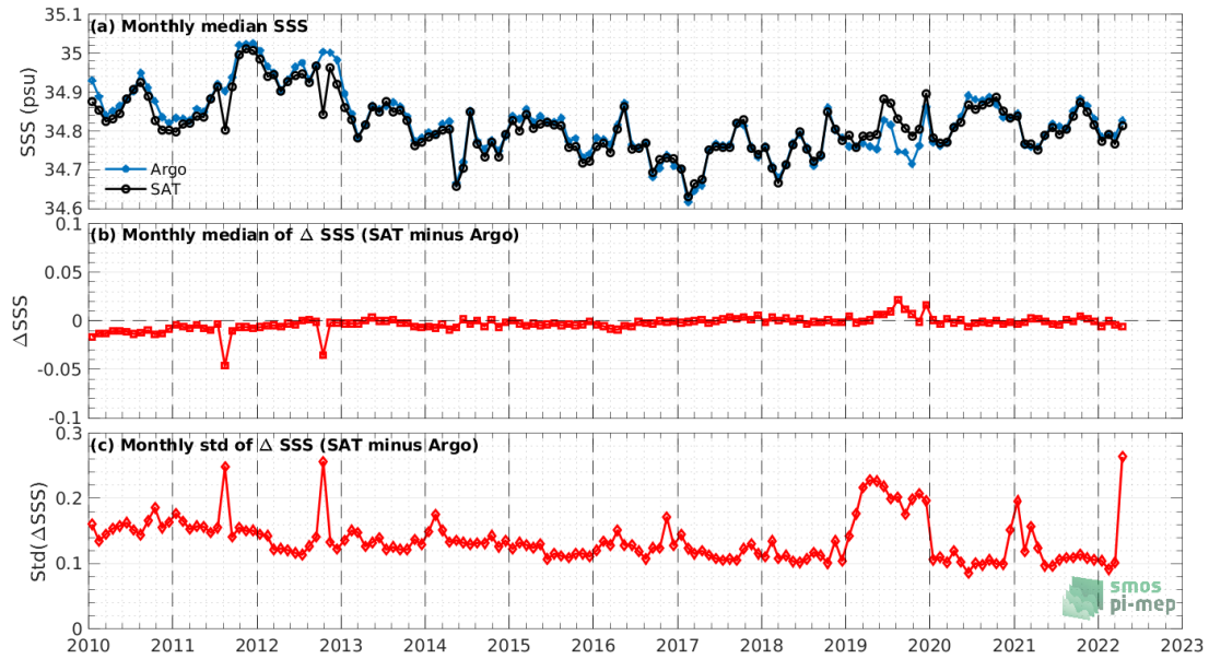
Figure 7: Time series of the monthly median SSS (top), median of \Delta SSS (Satellite - Argo) and Std of \Delta SSS (Satellite - Argo) over the Tropical Pacific Ocean Pi-MEP region considering all match-ups collected by the Pi-MEP.
