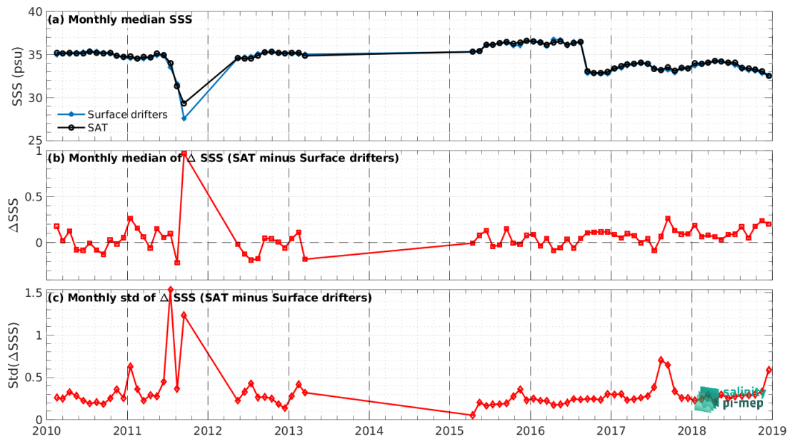
Figure 7: Time series of the monthly median SSS (top), median of \Delta SSS (Satellite - Surface drifters) and Std of \Delta SSS (Satellite - Surface drifters) over the Tropical Pacific Ocean Pi-MEP region considering all match-ups collected by the Pi-MEP.
