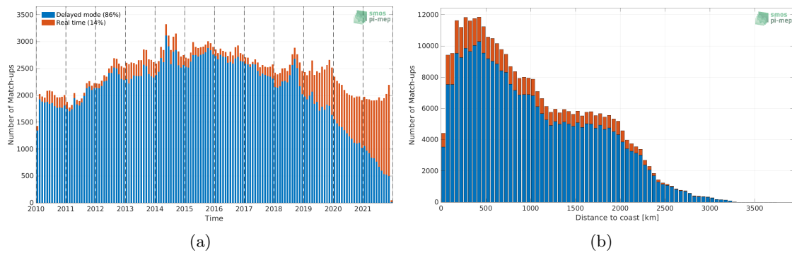
Figure 1: Number of match-ups between Argo and SMOS SSS L3 v7 - 18 Days (CATDS-CECOS-LOCEAN) SSS as a function of time (a) and as function of the distance to coast (b) over the Tropical Pacific Ocean Pi-MEP region and for the full satellite product period.
