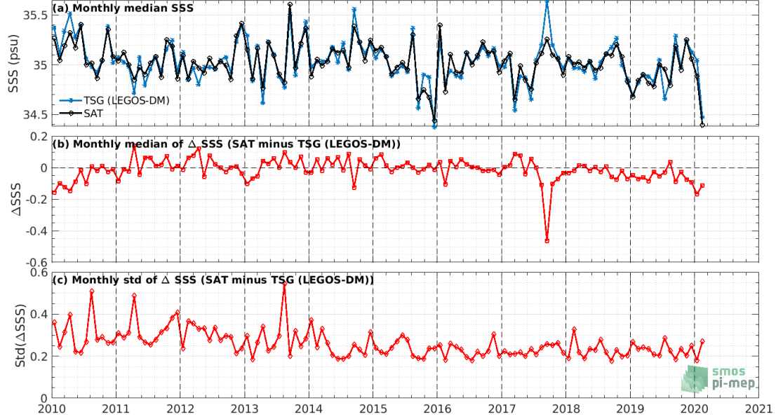
Figure 7: Time series of the monthly median SSS (top), median of \Delta\text{SSS} (Satellite - TSG (LEGOS-DM)) and Std of \Delta\text{SSS} (Satellite - TSG (LEGOS-DM)) over the Tropical Pacific Ocean Pi-MEP region considering all match-ups collected by the Pi-MEP.
