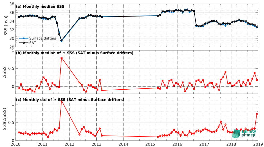
Figure 6: Time series of the monthly median SSS (top), median of \Delta SSS (Satellite - Surface drifters) and Std of \Delta SSS (Satellite - Surface drifters) over the Tropical Pacific Ocean Pi-MEP region considering all match-ups collected by the Pi-MEP.
