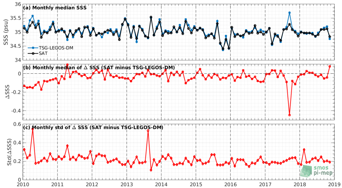
Figure 7: Time series of the monthly median SSS (top), median of \Delta SSS (Satellite - TSG-LEGOS-DM) and Std of \Delta SSS (Satellite - TSG-LEGOS-DM) over the Tropical Pacific Ocean Pi-MEP region considering all match-ups collected by the Pi-MEP.
