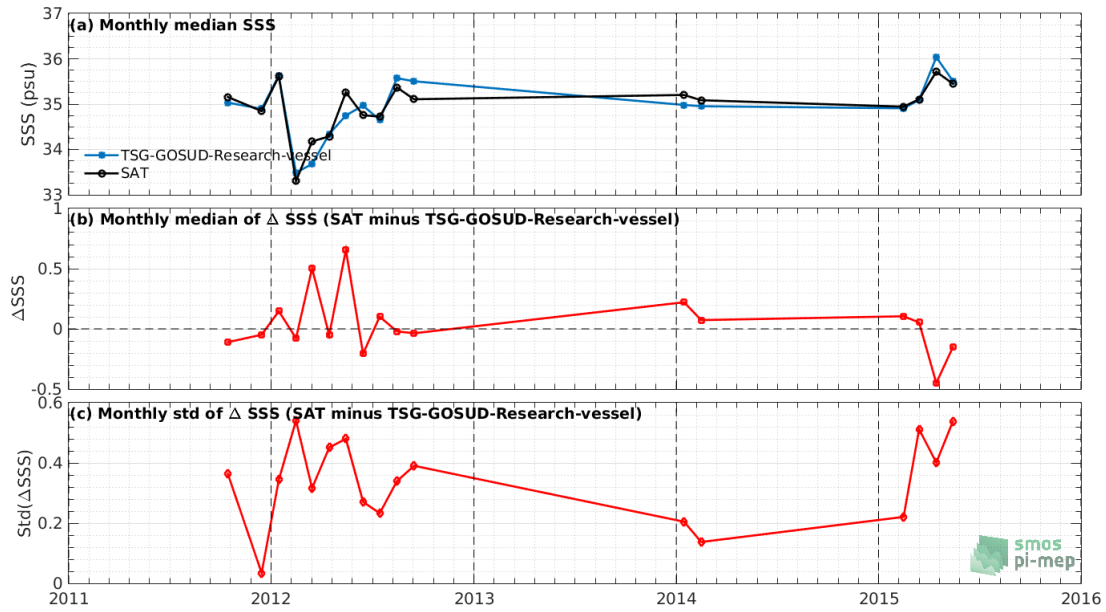
Figure 7: Time series of the monthly median SSS (top), median of \Delta SSS (Satellite - TSG-GOSUD-Research-vessel) and Std of \Delta SSS (Satellite - TSG-GOSUD-Research-vessel) over the Tropical Pacific Ocean Pi-MEP region considering all match-ups collected by the Pi-MEP.
