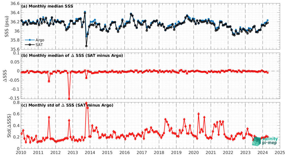
Figure 8: Time series of the monthly median SSS (top), median of \Delta SSS (Satellite - Argo) and Std of \Delta SSS (Satellite - Argo) over the Tropical Atlantic Ocean Pi-MEP region considering all match-ups collected by the Pi-MEP.
