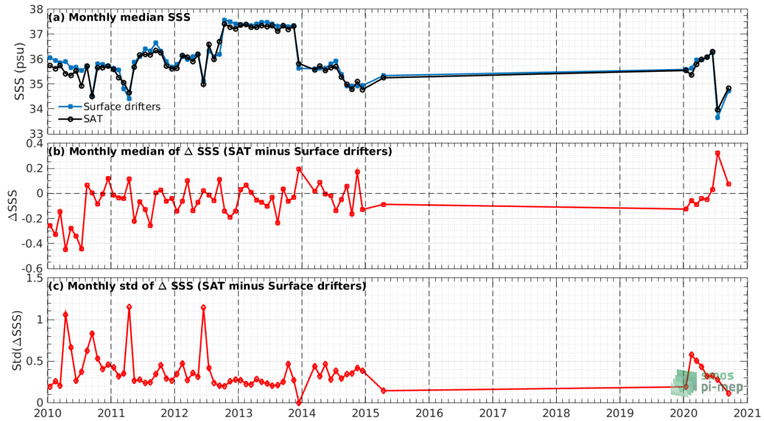
Figure 6: Time series of the monthly median SSS (top), median of \Delta SSS (Satellite - Surface drifters) and Std of \Delta SSS (Satellite - Surface drifters) over the Tropical Atlantic Ocean Pi-MEP region considering all match-ups collected by the Pi-MEP.
