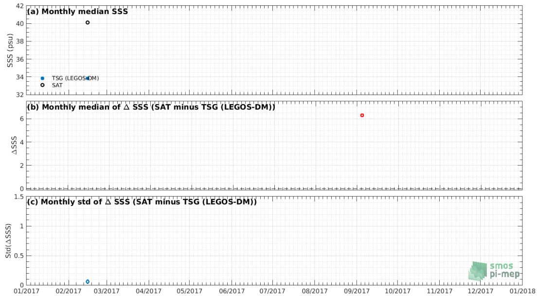
Figure 7: Time series of the monthly median SSS (top), median of \Delta SSS (Satellite - TSG (LEGOS-DM)) and Std of \Delta SSS (Satellite - TSG (LEGOS-DM)) over the Sea of Japan Pi-MEP region considering all match-ups collected by the Pi-MEP.
