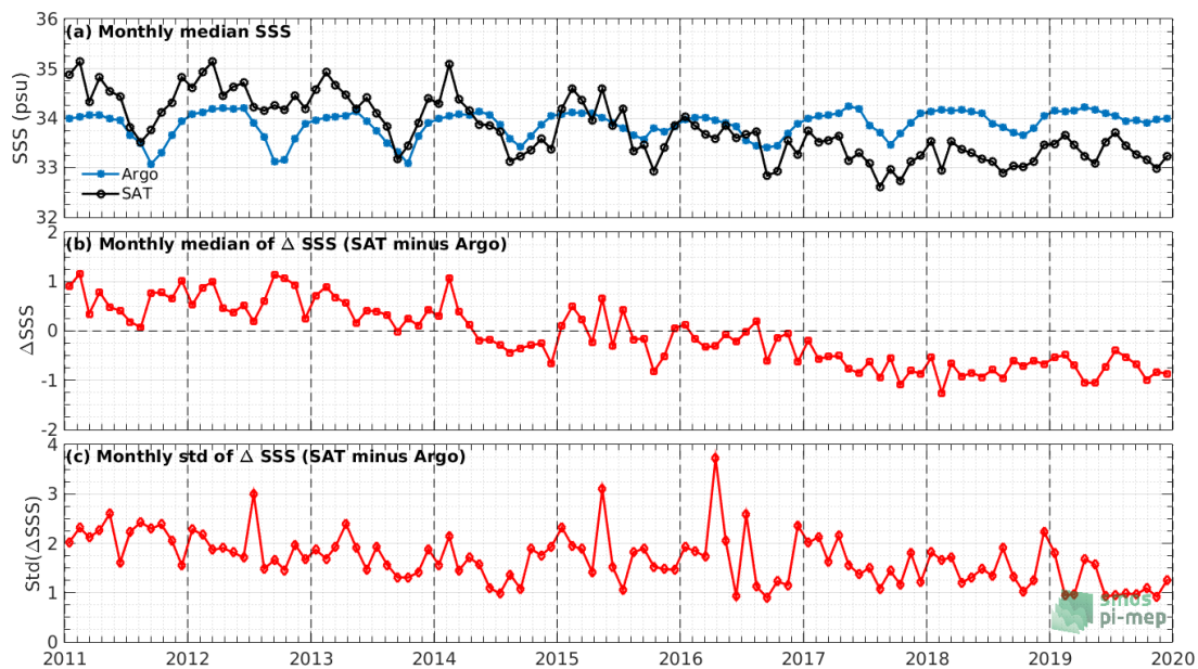
Figure 7: Time series of the monthly median SSS (top), median of \Delta SSS (Satellite - Argo) and Std of \Delta SSS (Satellite - Argo) over the Sea of Japan Pi-MEP region considering all match-ups collected by the Pi-MEP.
