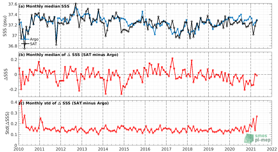
Figure 7: Time series of the monthly median SSS (top), median of \Delta SSS (Satellite - Argo) and Std of \Delta SSS (Satellite - Argo) over the SPURS 1 Pi-MEP region considering all match-ups collected by the Pi-MEP.
