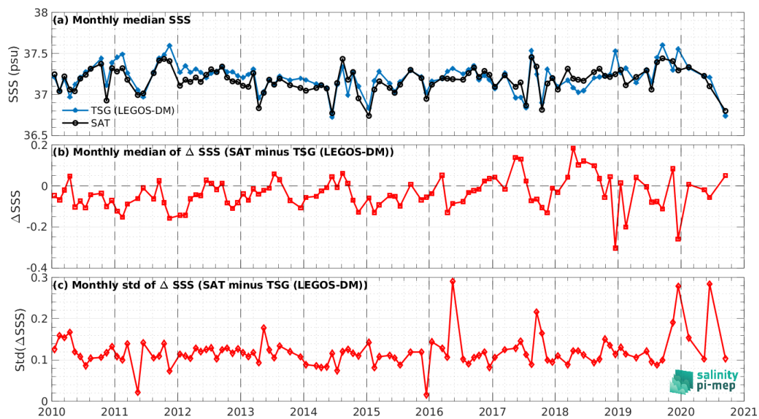
Figure 7: Time series of the monthly median SSS (top), median of \Delta SSS (Satellite - TSG (LEGOS-DM)) and Std of \Delta SSS (Satellite - TSG (LEGOS-DM)) over the SPURS 1 Pi-MEP region considering all match-ups collected by the Pi-MEP.
