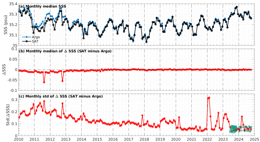
Figure 8: Time series of the monthly median SSS (top), median of \Delta SSS (Satellite - Argo) and Std of \Delta SSS (Satellite - Argo) over the South Pacific Ocean Pi-MEP region considering all match-ups collected by the Pi-MEP.
