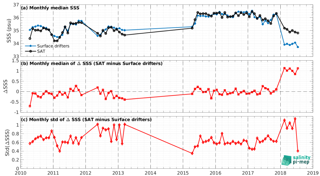
Figure 7: Time series of the monthly median SSS (top), median of \Delta SSS (Satellite - Surface drifters) and Std of \Delta SSS (Satellite - Surface drifters) over the South Pacific Ocean Pi-MEP region considering all match-ups collected by the Pi-MEP.
