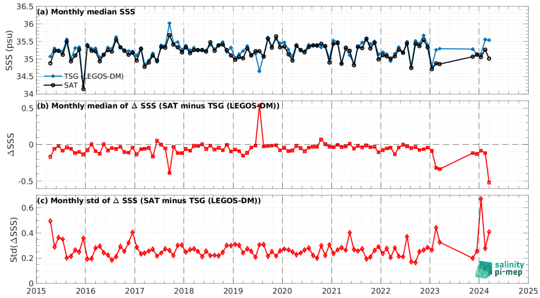
Figure 8: Time series of the monthly median SSS (top), median of \Delta SSS (Satellite - TSG (LEGOS-DM)) and Std of \Delta SSS (Satellite - TSG (LEGOS-DM)) over the South Pacific Ocean Pi-MEP region considering all match-ups collected by the Pi-MEP.
