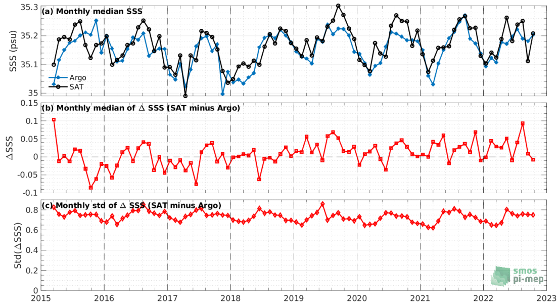
Figure 7: Time series of the monthly median SSS (top), median of \Delta SSS (Satellite - Argo) and Std of \Delta SSS (Satellite - Argo) over the South Pacific Ocean Pi-MEP region considering all match-ups collected by the Pi-MEP.
