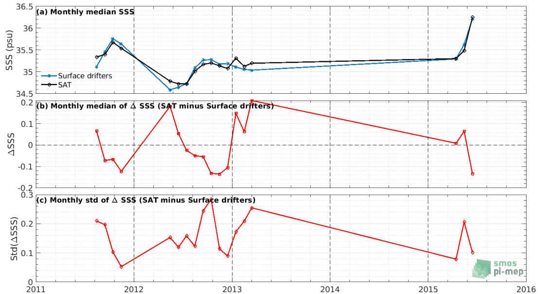
Figure 6: Time series of the monthly median SSS (top), median of \Delta SSS (Satellite - Surface drifters) and Std of \Delta SSS (Satellite - Surface drifters) over the South Pacific Ocean Pi-MEP region considering all match-ups collected by the Pi-MEP.
