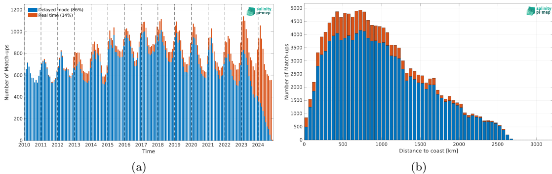
Figure 2: Number of match-ups between Argo and SMOS SSS L4 v1 - Monthly (CMEMS-CNR) SSS as a function of time (a) and as function of the distance to coast (b) over the Southern Ocean Pi-MEP region and for the full satellite product period.
