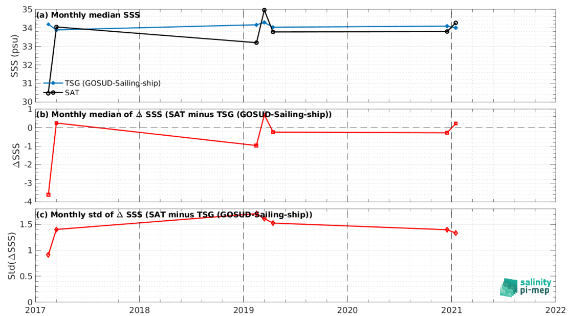
Figure 8: Time series of the monthly median SSS (top), median of \Delta SSS (Satellite - TSG (GOSUD-Sailing-ship)) and Std of \Delta SSS (Satellite - TSG (GOSUD-Sailing-ship)) over the Southern Ocean Pi-MEP region considering all match-ups collected by the Pi-MEP.
