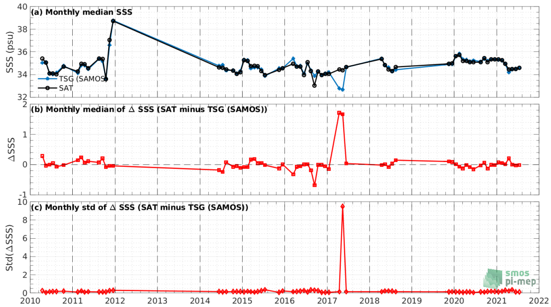
Figure 7: Time series of the monthly median SSS (top), median of \Delta SSS (Satellite - TSG (SAMOS)) and Std of \Delta SSS (Satellite - TSG (SAMOS)) over the SMOS coastal zone (<800km) 60N-60S Pi-MEP region considering all match-ups collected by the Pi-MEP.
