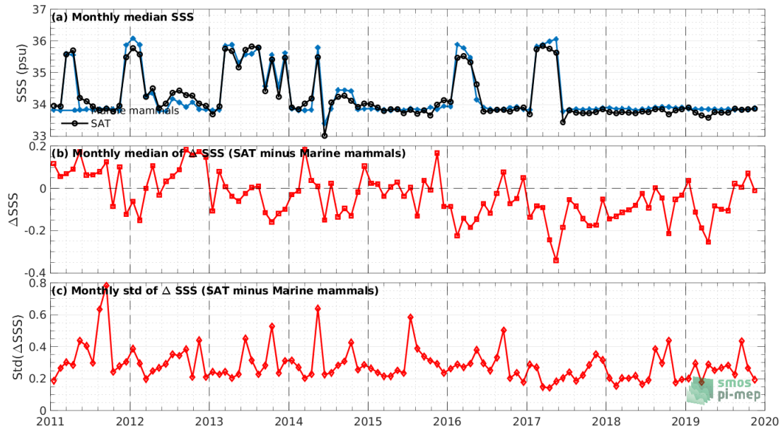
Figure 7: Time series of the monthly median SSS (top), median of \Delta SSS (Satellite - Marine mammals) and Std of \Delta SSS (Satellite - Marine mammals) over the SMOS coastal zone (<800km) 60N-60S Pi-MEP region considering all match-ups collected by the Pi-MEP.
