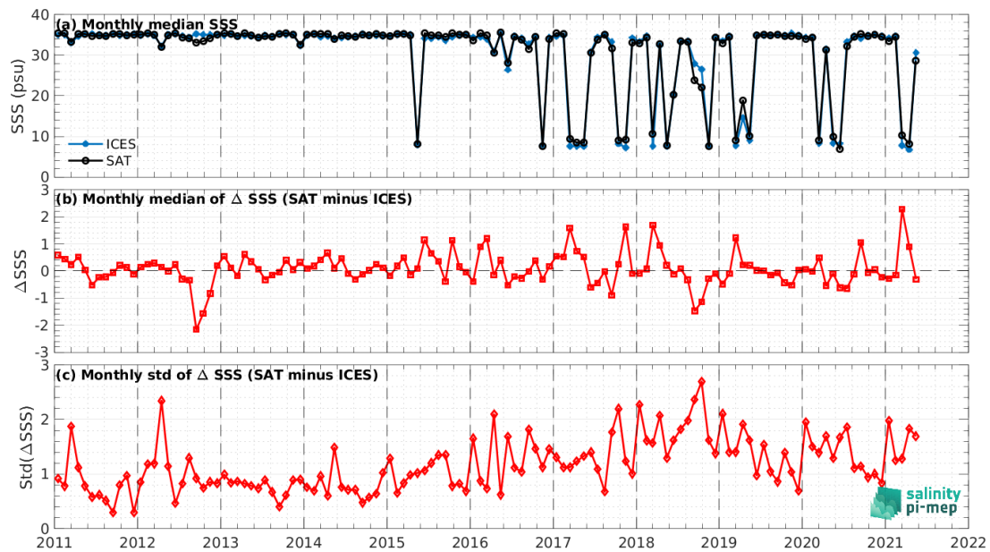
Figure 8: Time series of the monthly median SSS (top), median of \Delta SSS (Satellite - ICES) and Std of \Delta SSS (Satellite - ICES) over the SMOS coastal zone (<800km) 60N-60S Pi-MEP region considering all match-ups collected by the Pi-MEP.
