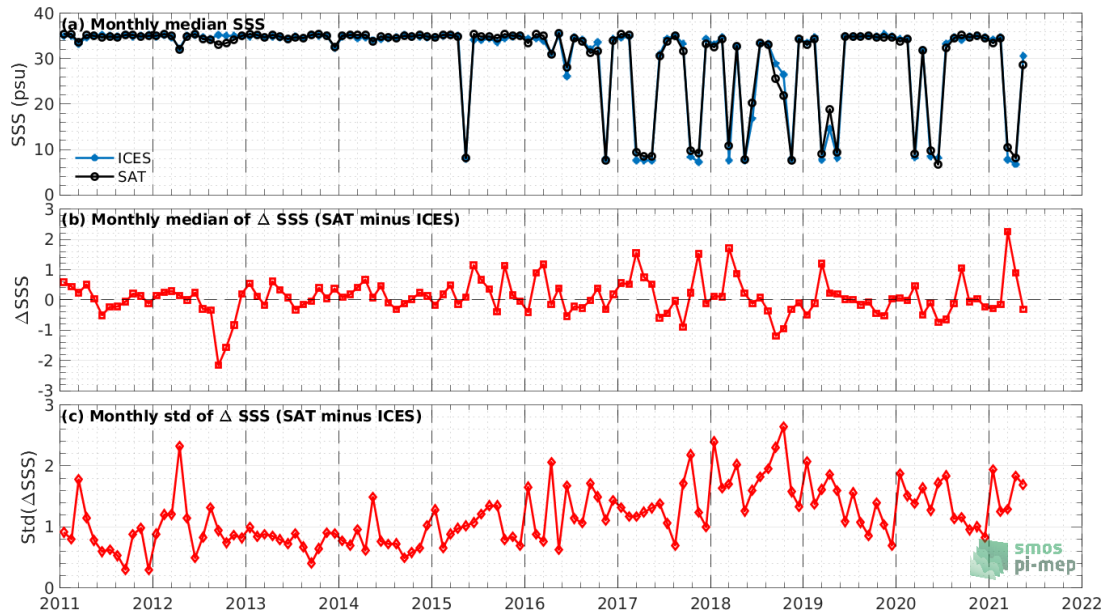
Figure 7: Time series of the monthly median SSS (top), median of \Delta SSS (Satellite - ICES) and Std of \Delta SSS (Satellite - ICES) over the SMOS coastal zone (<800km) 60N-60S Pi-MEP region considering all match-ups collected by the Pi-MEP.
