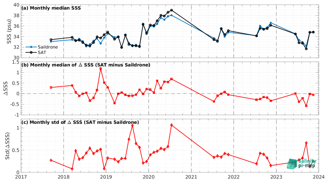
Figure 8: Time series of the monthly median SSS (top), median of \Delta SSS (Satellite - Sairdrone) and Std of \Delta SSS (Satellite - Sairdrone) over the SMOS coastal zone ( <800\text{km} ) 60\text{N} - 60\text{S} Pi-MEP region considering all match-ups collected by the Pi-MEP.
