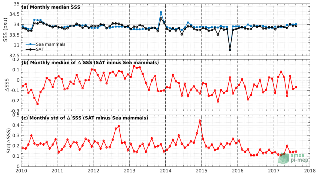
Figure 7: Time series of the monthly median SSS (top), median of \Delta SSS (Satellite - Sea mammals) and Std of \Delta SSS (Satellite - Sea mammals) over the SMOS coastal zone (<800km) 60N-60S Pi-MEP region considering all match-ups collected by the Pi-MEP.
