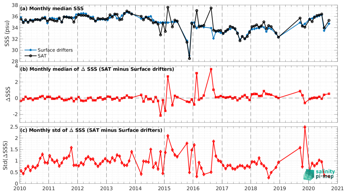
Figure 7: Time series of the monthly median SSS (top), median of \Delta SSS (Satellite - Surface drifters) and Std of \Delta SSS (Satellite - Surface drifters) over the SMOS coastal zone (<800km) 60N-60S Pi-MEP region considering all match-ups collected by the Pi-MEP.
