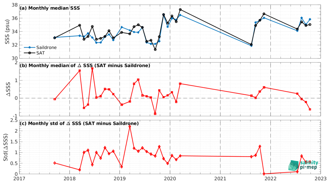
Figure 7: Time series of the monthly median SSS (top), median of \Delta SSS (Satellite - Saildrone) and Std of \Delta SSS (Satellite - Saildrone) over the SMOS coastal zone (<800km) 60N-60S Pi-MEP region considering all match-ups collected by the Pi-MEP.
