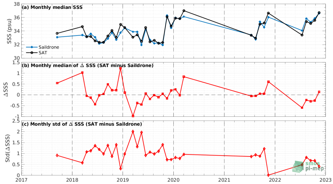
Figure 7: Time series of the monthly median SSS (top), median of \Delta SSS (Satellite - Sairdrone) and Std of \Delta SSS (Satellite - Sairdrone) over the SMOS coastal zone (<800km) 60N-60S Pi-MEP region considering all match-ups collected by the Pi-MEP.
