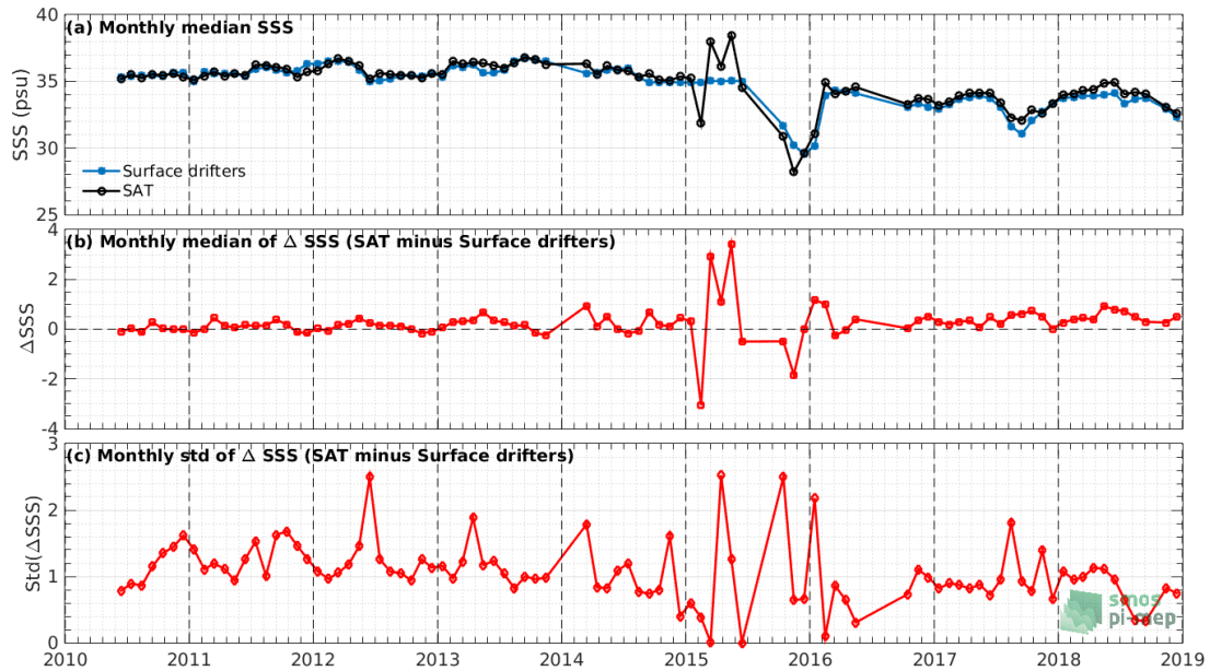
Figure 6: Time series of the monthly median SSS (top), median of \Delta SSS (Satellite - Surface drifters) and Std of \Delta SSS (Satellite - Surface drifters) over the SMOS coastal zone ( <800\text{km} ) 60N-60S Pi-MEP region considering all match-ups collected by the Pi-MEP.
