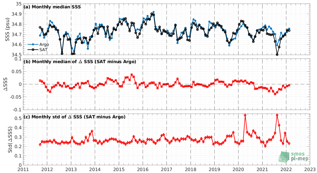
Figure 7: Time series of the monthly median SSS (top), median of \Delta SSS (Satellite - Argo) and Std of \Delta SSS (Satellite - Argo) over the SMOS coastal zone (<800km) 60N-60S Pi-MEP region considering all match-ups collected by the Pi-MEP.
