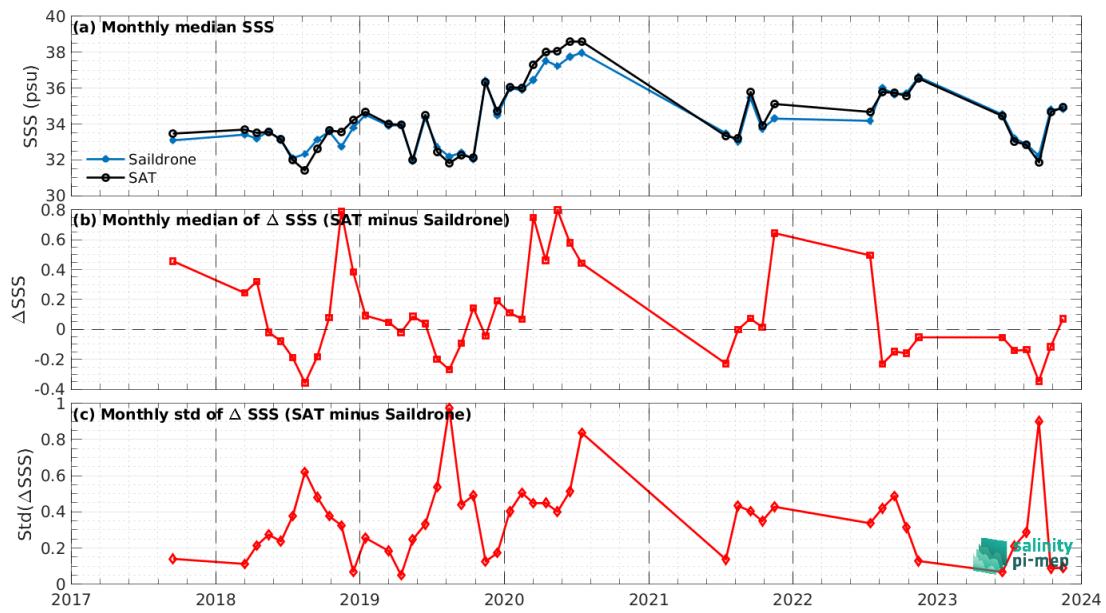
Figure 8: Time series of the monthly median SSS (top), median of \Delta SSS (Satellite - Saildrone) and Std of \Delta SSS (Satellite - Saildrone) over the SMOS coastal zone (<800km) 60N-60S Pi-MEP region considering all match-ups collected by the Pi-MEP.
