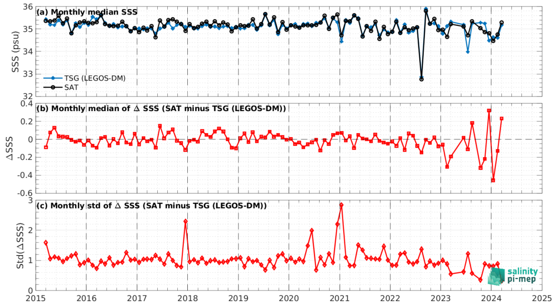
Figure 8: Time series of the monthly median SSS (top), median of \Delta SSS (Satellite - TSG (LEGOS-DM)) and Std of \Delta SSS (Satellite - TSG (LEGOS-DM)) over the SMOS coastal zone (<800km) 60N-60S Pi-MEP region considering all match-ups collected by the Pi-MEP.
