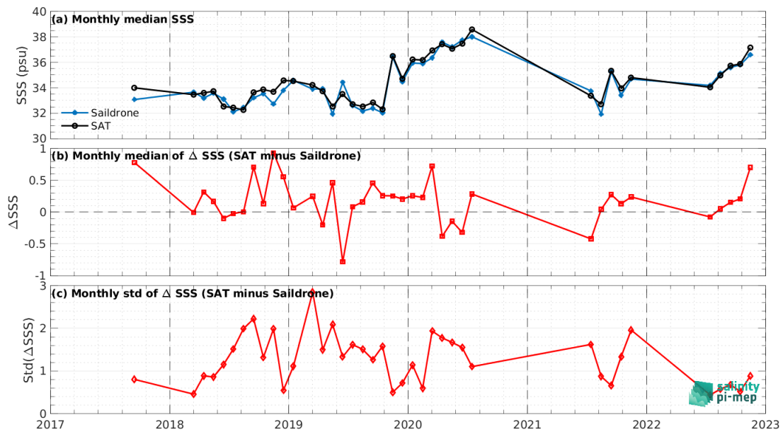
Figure 7: Time series of the monthly median SSS (top), median of \Delta SSS (Satellite - Saildrone) and Std of \Delta SSS (Satellite - Saildrone) over the SMOS coastal zone ( <800\text{km} ) 60\text{N} - 60\text{S} Pi-MEP region considering all match-ups collected by the Pi-MEP.
