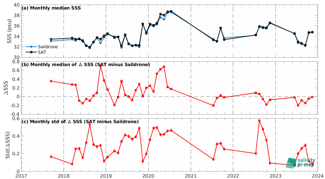
Figure 8: Time series of the monthly median SSS (top), median of \Delta SSS (Satellite - Saildrone) and Std of \Delta SSS (Satellite - Saildrone) over the SMOS coastal zone ( <800\text{km} ) 60N-60S Pi-MEP region considering all match-ups collected by the Pi-MEP.
