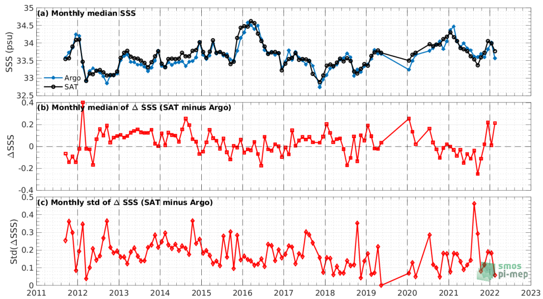
Figure 7: Time series of the monthly median SSS (top), median of \Delta SSS (Satellite - Argo) and Std of \Delta SSS (Satellite - Argo) over the South China Sea Pi-MEP region considering all match-ups collected by the Pi-MEP.
