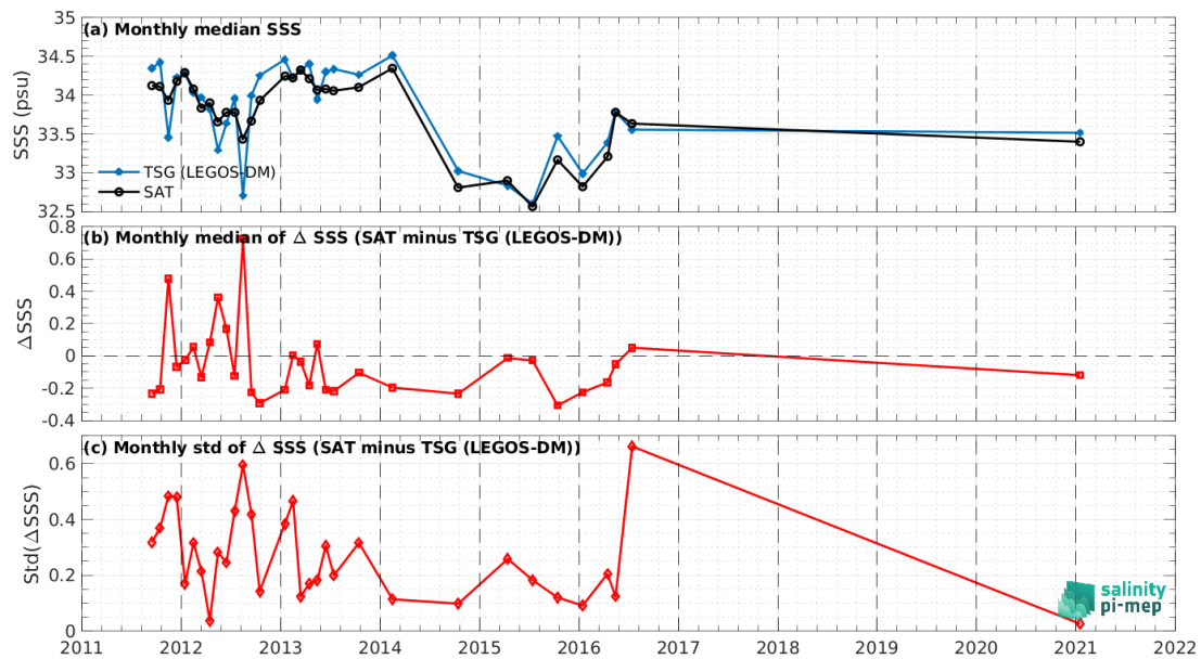
Figure 8: Time series of the monthly median SSS (top), median of \Delta SSS (Satellite - TSG (LEGOS-DM)) and Std of \Delta SSS (Satellite - TSG (LEGOS-DM)) over the South China Sea Pi-MEP region considering all match-ups collected by the Pi-MEP.
