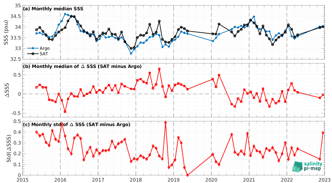
Figure 8: Time series of the monthly median SSS (top), median of \Delta SSS (Satellite - Argo) and Std of \Delta SSS (Satellite - Argo) over the South China Sea Pi-MEP region considering all match-ups collected by the Pi-MEP.
