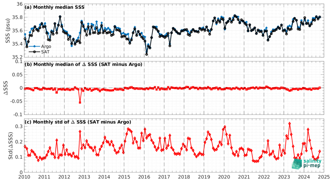
Figure 8: Time series of the monthly median SSS (top), median of \Delta SSS (Satellite - Argo) and Std of \Delta SSS (Satellite - Argo) over the South Atlantic Ocean Pi-MEP region considering all match-ups collected by the Pi-MEP.
