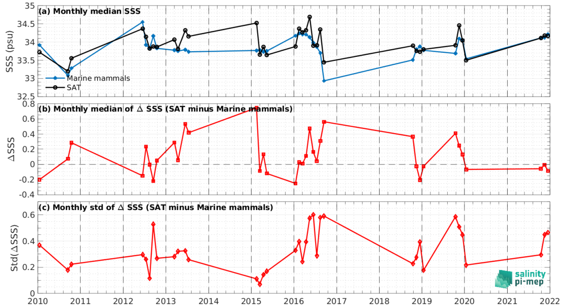
Figure 8: Time series of the monthly median SSS (top), median of \Delta SSS (Satellite - Marine mammals) and Std of \Delta SSS (Satellite - Marine mammals) over the South Atlantic Ocean Pi-MEP region considering all match-ups collected by the Pi-MEP.
