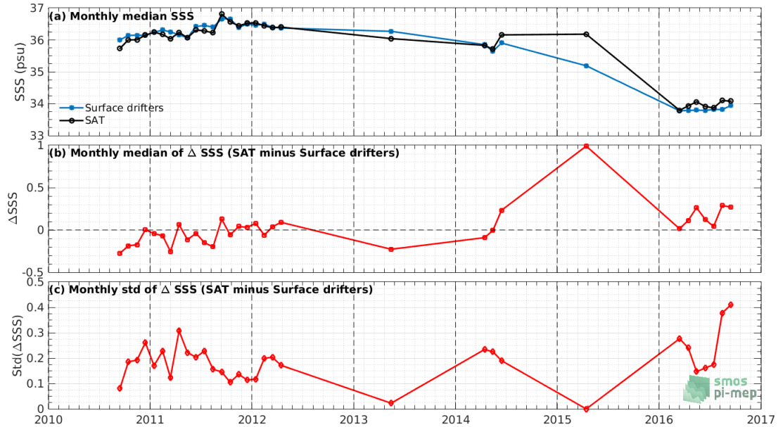
Figure 6: Time series of the monthly median SSS (top), median of \Delta SSS (Satellite - Surface drifters) and Std of \Delta SSS (Satellite - Surface drifters) over the South Atlantic Ocean Pi-MEP region considering all match-ups collected by the Pi-MEP.
