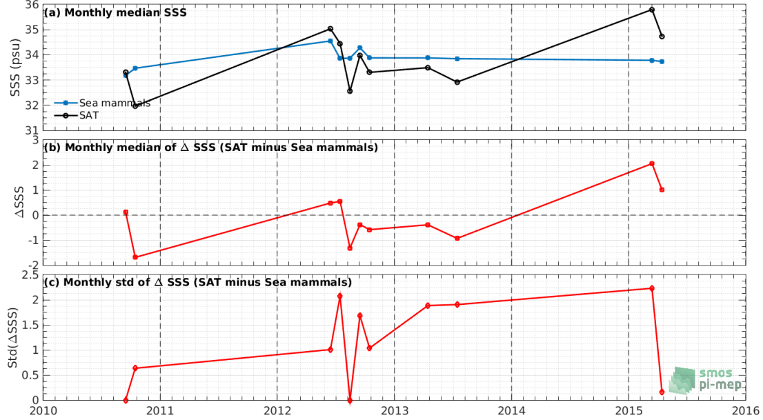
Figure 7: Time series of the monthly median SSS (top), median of \Delta SSS (Satellite - Sea mammals) and Std of \Delta SSS (Satellite - Sea mammals) over the South Atlantic Ocean Pi-MEP region considering all match-ups collected by the Pi-MEP.
