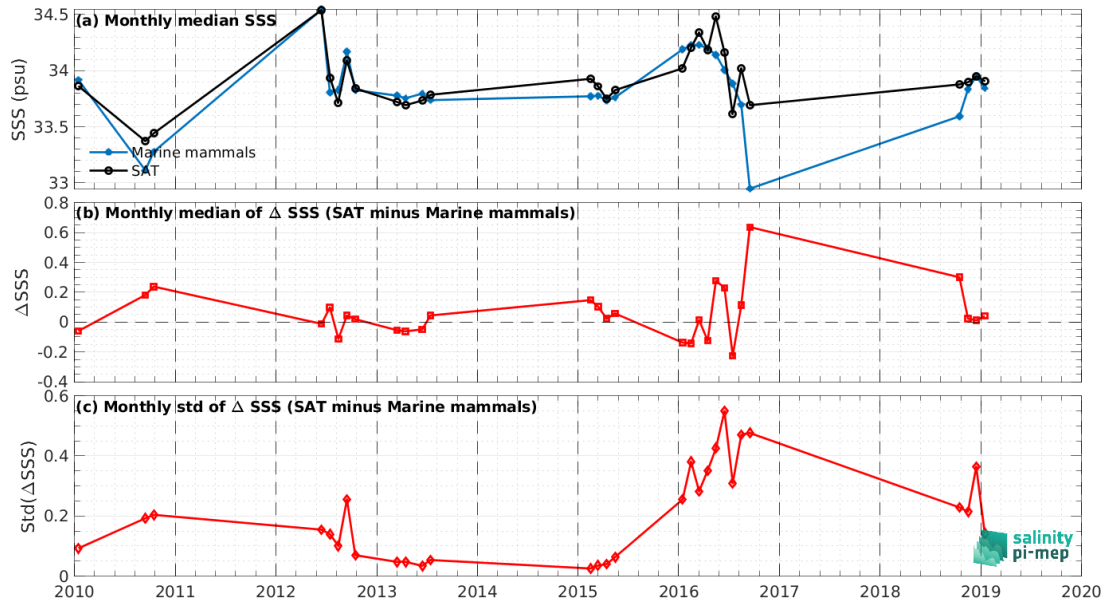
Figure 7: Time series of the monthly median SSS (top), median of \Delta SSS (Satellite - Marine mammals) and Std of \Delta SSS (Satellite - Marine mammals) over the South Atlantic Ocean Pi-MEP region considering all match-ups collected by the Pi-MEP.
