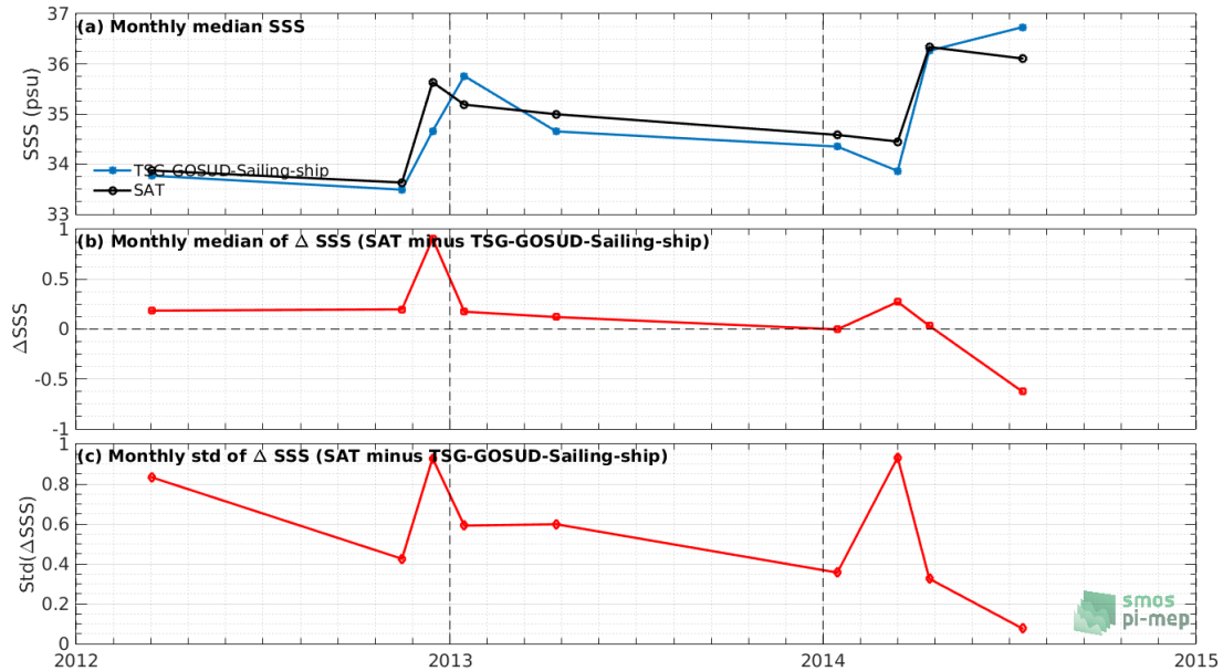
Figure 7: Time series of the monthly median SSS (top), median of \Delta SSS (Satellite - TSG-GOSUD-Sailing-ship) and Std of \Delta SSS (Satellite - TSG-GOSUD-Sailing-ship) over the South Atlantic Ocean Pi-MEP region considering all match-ups collected by the Pi-MEP.
