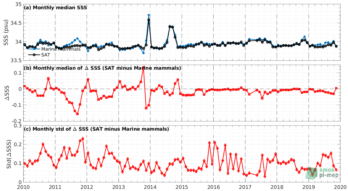
Figure 7: Time series of the monthly median SSS (top), median of \Delta SSS (Satellite - Marine mammals) and Std of \Delta SSS (Satellite - Marine mammals) over the Roaring Forties and Furious Fifties Pi-MEP region considering all match-ups collected by the Pi-MEP.
