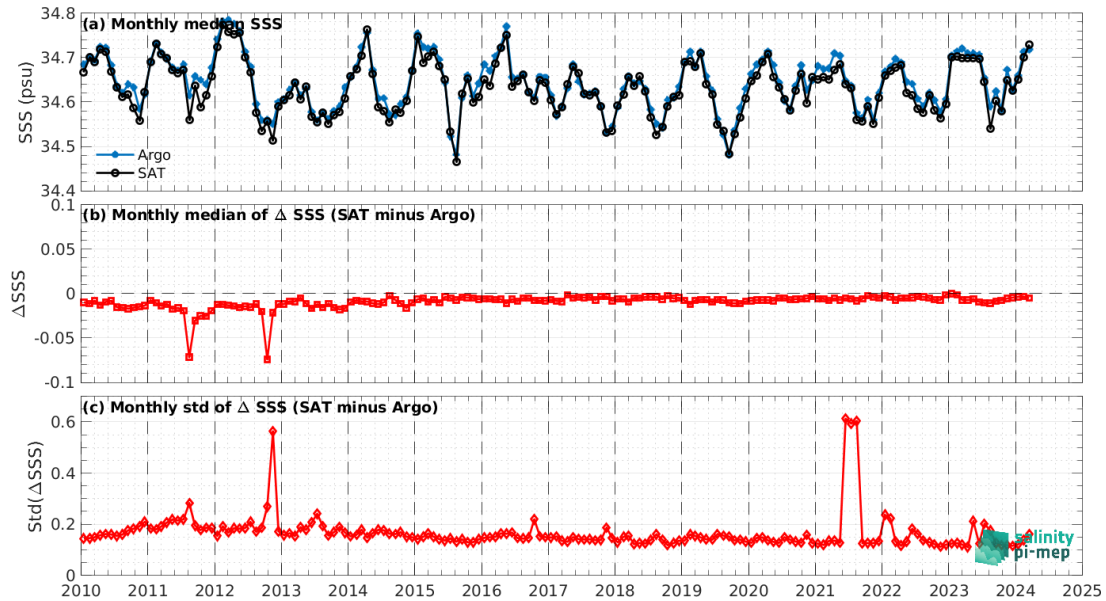
Figure 8: Time series of the monthly median SSS (top), median of \Delta SSS (Satellite - Argo) and Std of \Delta SSS (Satellite - Argo) over the Pacific Ocean Pi-MEP region considering all match-ups collected by the Pi-MEP.
