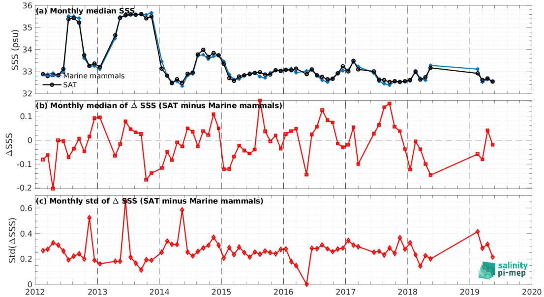
Figure 7: Time series of the monthly median SSS (top), median of \Delta\text{SSS} (Satellite - Marine mammals) and Std of \Delta\text{SSS} (Satellite - Marine mammals) over the Pacific Ocean Pi-MEP region considering all match-ups collected by the Pi-MEP.
