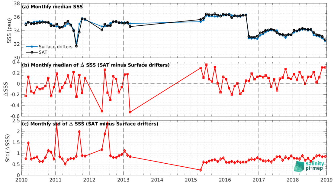
Figure 7: Time series of the monthly median SSS (top), median of \Delta SSS (Satellite - Surface drifters) and Std of \Delta SSS (Satellite - Surface drifters) over the Pacific Ocean Pi-MEP region considering all match-ups collected by the Pi-MEP.
