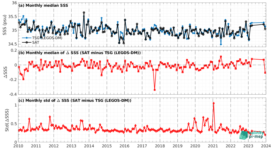
Figure 8: Time series of the monthly median SSS (top), median of \Delta SSS (Satellite - TSG (LEGOS-DM)) and Std of \Delta SSS (Satellite - TSG (LEGOS-DM)) over the Pacific Ocean Pi-MEP region considering all match-ups collected by the Pi-MEP.
