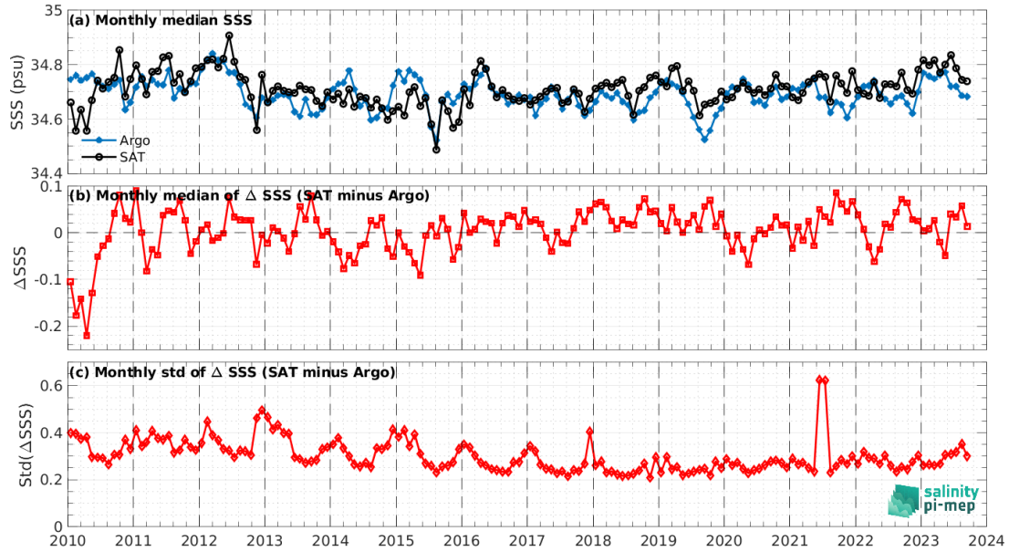
Figure 7: Time series of the monthly median SSS (top), median of \Delta SSS (Satellite - Argo) and Std of \Delta SSS (Satellite - Argo) over the Pacific Ocean Pi-MEP region considering all match-ups collected by the Pi-MEP.
